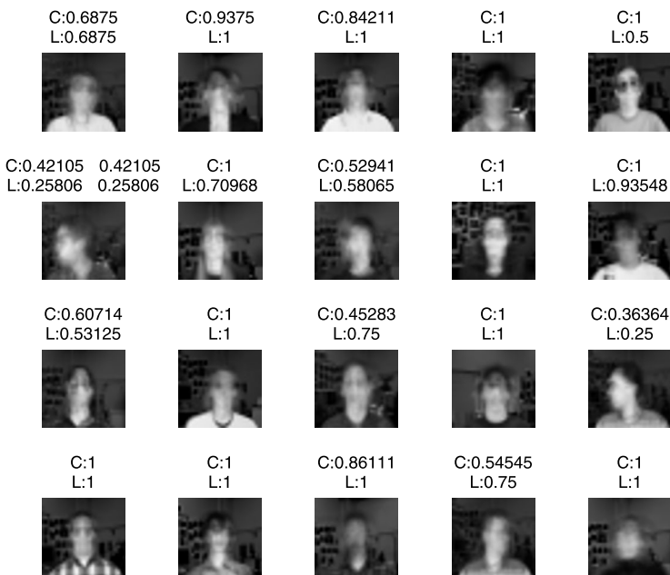
Fig. 5 Average images for 20 clusters generated by the first iteration of the algorithm using the standard inner product version (linear kernel) for the CMUFace dataset. Each image correspond to a different individual. Values above each image indicate the percentage of the individual's images inside the cluster (L value) and the percentage of the individual's images inside the specified cluster
