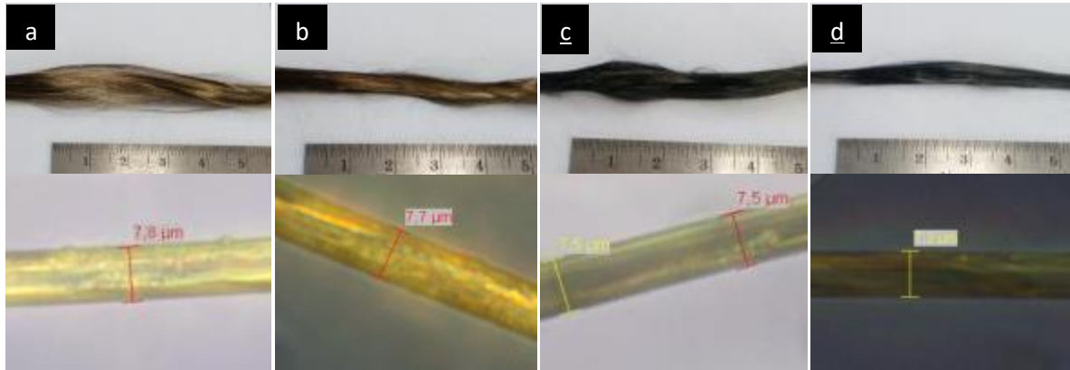
Figure 2. NiCF filaments: (a) before stripping; after stripping in (b) 37% HCl +3% H 2 O 2 (1:1); (c) 37% HCl +6% H 2 O 2 (1:1); (d) 37% HCl +10% H 2 O 2 (1:1). Rulers show main unit in cm.
