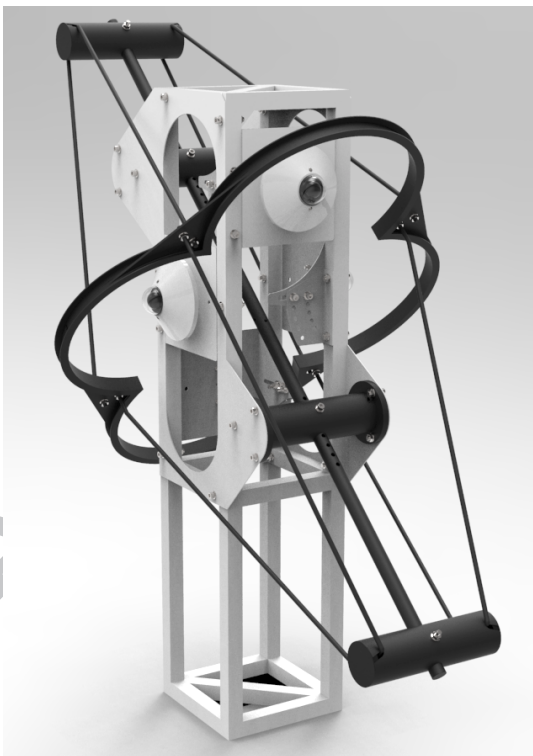
Fig. 3. Multi-directional diffuse solar irradiance measurement device aka MK6. Adapted from (de Simón-Martín et al., 2015).
