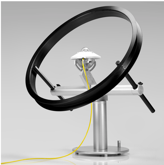
Fig. 2. Commercial Drummond's shadow-band device. Adapted from (Kipp and Zonen, 2014).
