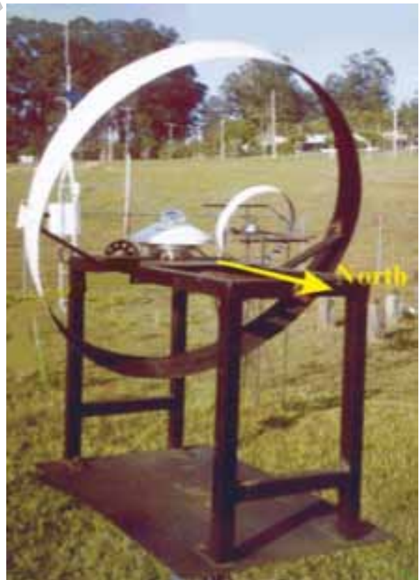
Figure 4: Oliveira's shadow-ring device [18].
