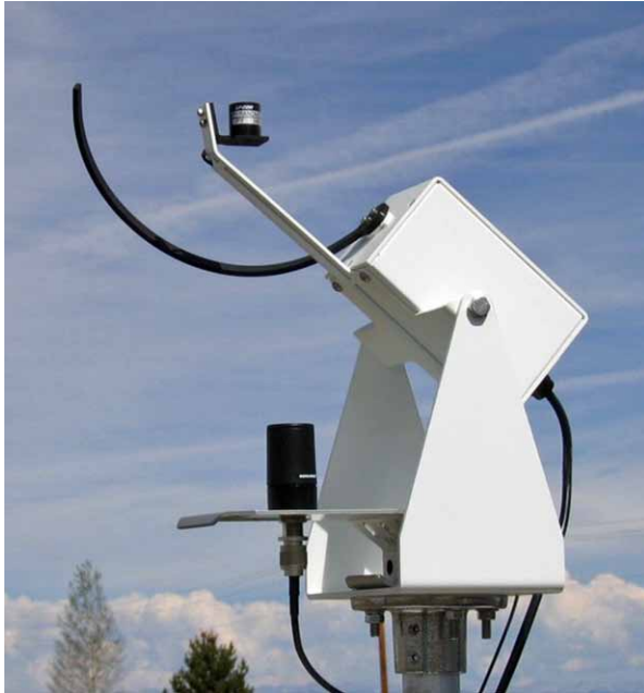
Figure 2: Commercial example of rotating shadowband [15].
