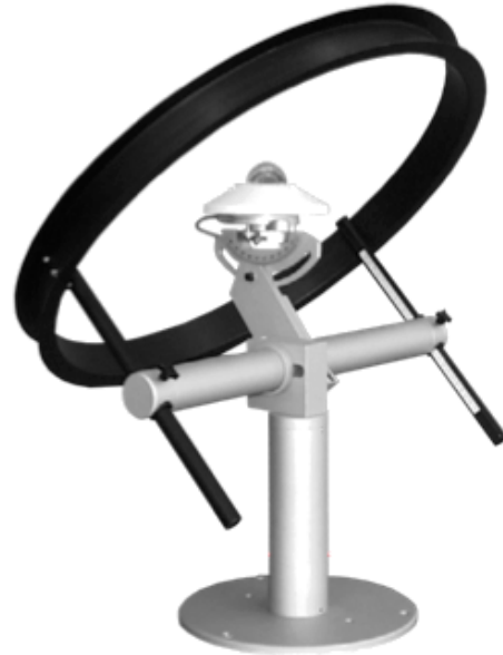
Figure 1: Commercial example of Drummond's shadow-ring [11].
