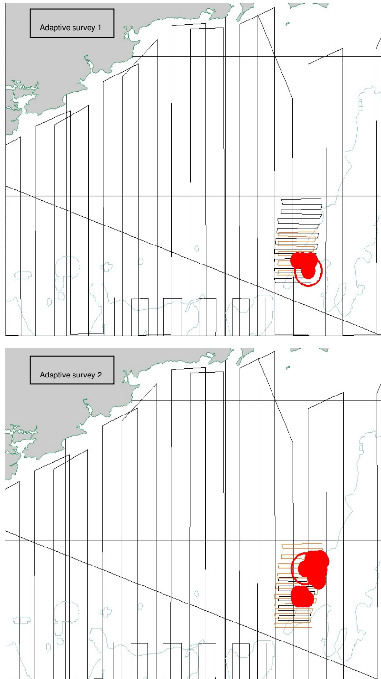
Figure 3. Herring NASC (Nautical area scattering coefficient) plot of the distribution from adaptive survey effort. Top Panel: adaptive Survey 1; bottom panel: adaptive Survey 2. Active transects shown in orange. Transects spacing is 1nmi
