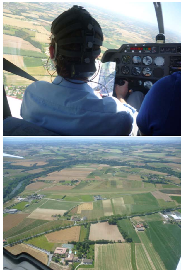
FIGURE 2 In-flight navigation to a grass airstrip. Top: Pilot (shown here wearing the Cognionics HD-72 dry-wireless 64 channel EEG system) looking at aeronautical charts to navigate to an airfield with a grass airstrip while simultaneously carrying out the audio task of responding by button press to audio alarm stimuli. Bottom: The grass airstrip (in the center of the image) can be quite difficult to see from the air. One needs to find landmarks on the aeronautical chart (e.g., a river) to help locate the grass airstrip amongst all the other green fields
