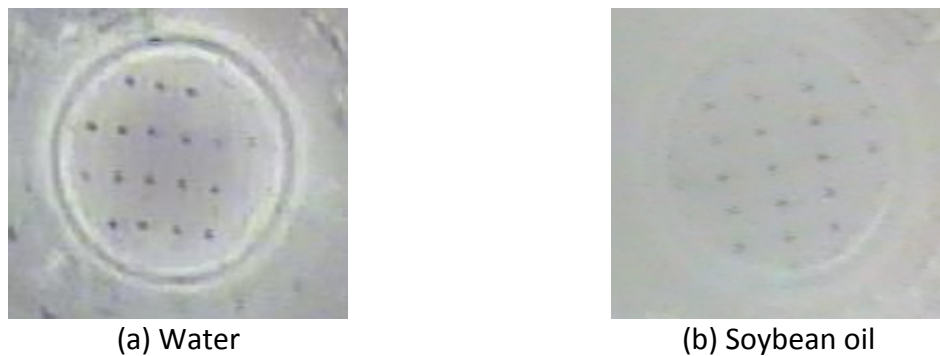
Figure 3.8: A 10 mm marker array filmed through 480 mm of water (a) and soybean oil (b) to assess the depth of field of the underwater cameras used in the buoyancy study.
