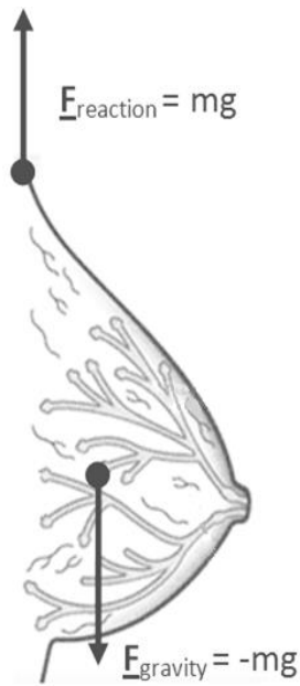
Figure 2.2: Misalignment of gravity and the ground reaction force acting on the breast.
