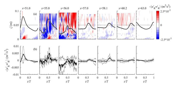
**Figure 7.** Phase-averaged turbulent Reynolds stress  $-\langle u'_R w'_R \rangle$ . (a) Depth-varying phase-dependent turbulent Reynolds stress (color contour), with the free-stream bed-parallel velocity  $\langle u_{R,\infty} \rangle$  (black line) for reference; (b) phase-averaged Reynolds stress at  $\zeta = 0.001$  m (black)  $\pm$  1 standard deviation (grey).
