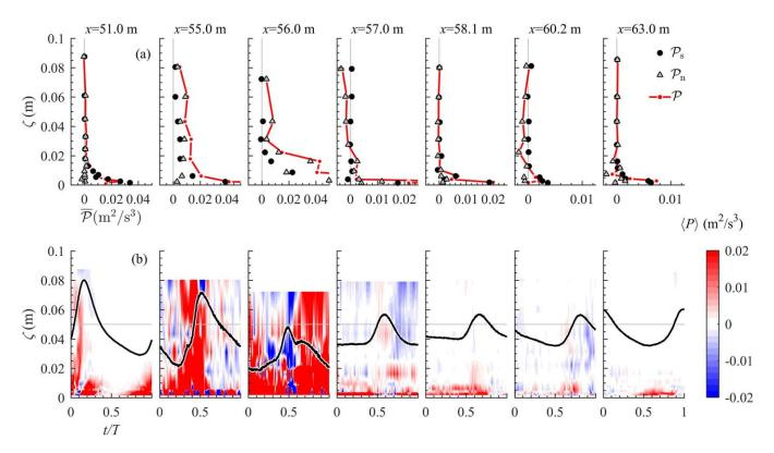
**Figure 8.** Turbulent production rates. (a) Time-averaged production, contribution by shear stresses (black diamond), contribution by normal stresses (grey triangle), and sum of both contributions (red dots and line; note the different scales for the horizontal axes); (b) Phase-averaged production  $\mathcal{P}$  as color contour, including free-stream bed-parallel velocity  $\langle u_{\rm R,\infty} \rangle$  (black line) and  $\langle u_{\rm R,\infty} \rangle = 0$  (grey line) for reference.
