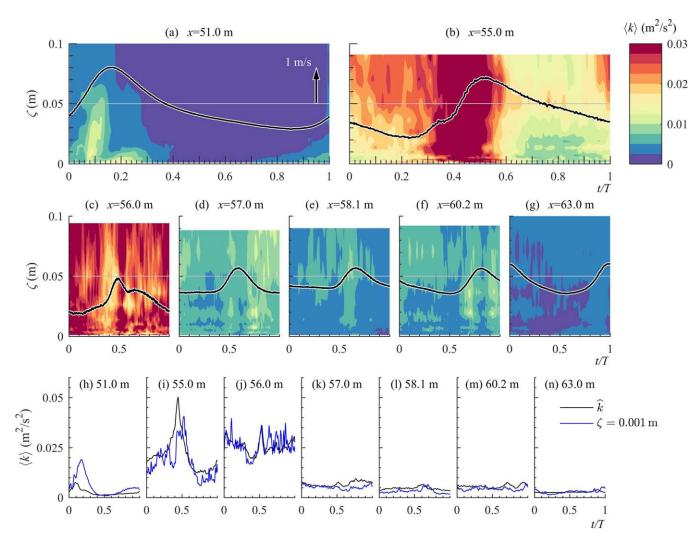
**Figure 5.** Time series of near-bed phase-averaged TKE. (a)–(g) depth-varying phase-dependent turbulent kinetic energy  $\langle k \rangle$  (color contour), with the free-stream bed-parallel velocity  $\langle u_{R,\infty} \rangle$  (black line) for reference (arrow in (a) indicates velocity magnitude); (h)–(n)  $\langle k \rangle$  at  $\zeta = 0.001$  m (blue) and depth-averaged over near-bed control volume (black).
