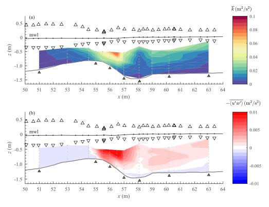
**Figure 4.** (a) Time-averaged turbulent kinetic energy; (b) time-averaged turbulent Reynolds stress. Open triangles at top mark maximum and minimum phase-averaged water surface. Grey dots indicate the outer-flow velocity measurement positions. Grey triangles at bottom mark the seven cross-shore locations for which detailed WBL velocities were measured.
