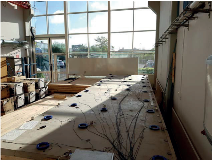
Figure 23. The concrete floor slab, used throughout the course of the thesis work. During the summer the sunlight raise the temperature in the room significantly and rapidly.
