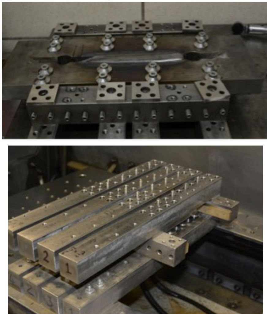
Figure 4: Clamping arrangement for contour method (EDM) cutting process. An NG-SAW test piece can be seen prior to (top) and after (bottom) fixing of the restraining bars.
