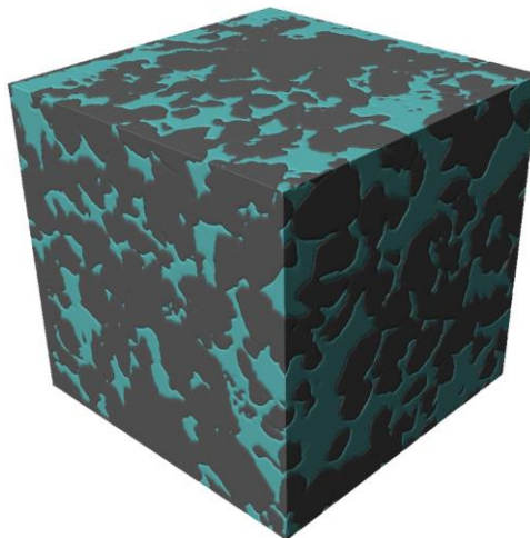
Fig. 1. Segmented micro-CT scan of a dry Berea sandstone sample (data source: [5])
