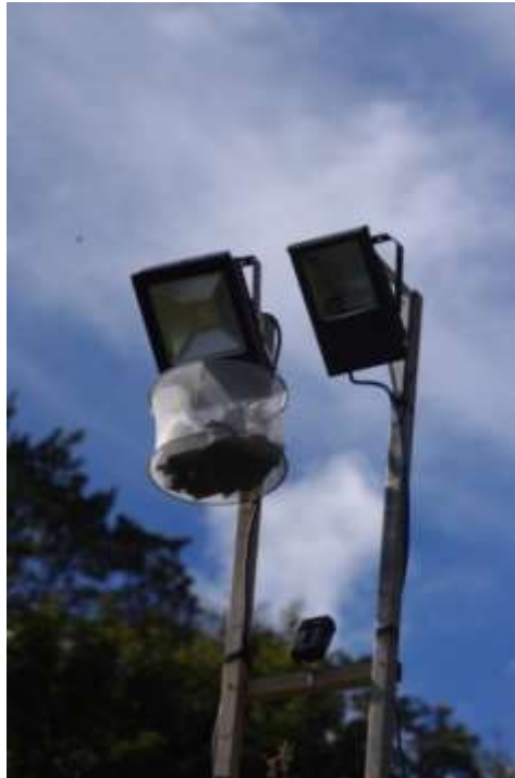
Figure A 3.2: Photograph of Safari moth trap suspended below one of the lamppost structures; lamps act as backboard, deflecting moths into the traps. The LED is on the left of the picture and the ceramic metal halide is on the right.
