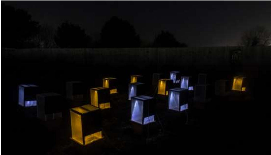
Figure 5.2: Photograph of experimental setup: The image depicts the block of 18 light cages(6 x white, 6 x amber and 6 x dark control cages), within which the oak saplings and winter moth ova were positioned. The dark panels on the sides of the illuminated cages prevent light spill into neighbouring cages; baffles along either side of the LED strips prevent light spill in the other direction.
