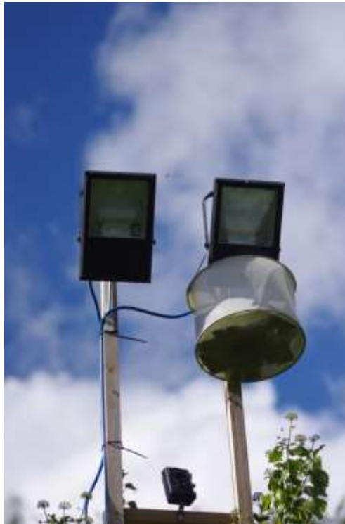
Figure A2.1: photograph of safari moth trap containing standardised amount of seedling trays, suspended from one of the lamppost structures.
