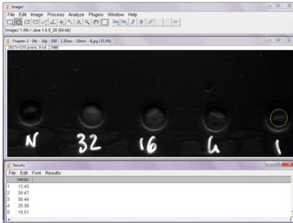
Figure 10 - Image analysis. A) Image of a paper-based device taken using a desktop scanner. B) Image transformed into grayscale. C) Image analysed with Image J, after image invert and after oval selection of the area to be measured. Results show measurement in mean grey value.
