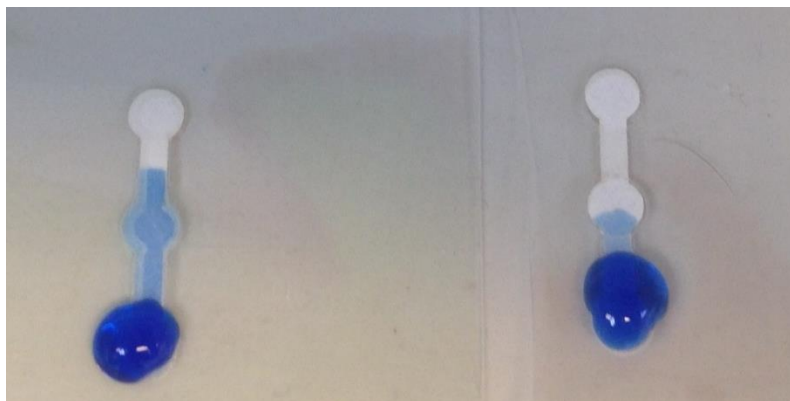
Figure 51 - Effect of lamination on the flow rate. On the left, the device has lamination that partially covers the paper cut-out. On the right, the device has lamination completely covering the microchannels and leaving the paper pads open. Picture taken 2 min after application of 50 \mu l food colouring in the reagents inlet.
