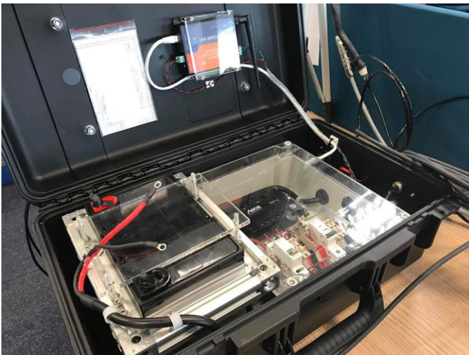
Figure 4: General design of the wireless water quality monitoring system
