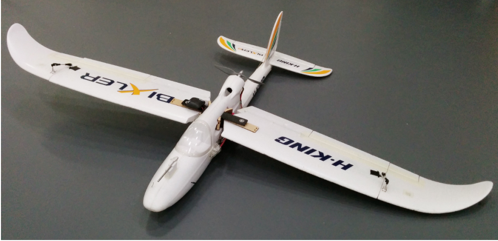
Figure 1: Bixler 2 Airframe, fitted with variable sweep and twist mechanisms
