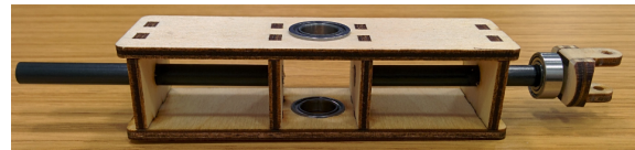
(c) Spar boxing for wing root
