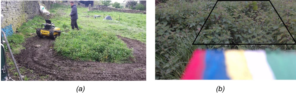
Figure 1: Training image acquisition (from [1]). (a) Plot of Urtica and ground robot (IBEX2) capturing training images from the plot using its on-board cameras. (b) Raw training image of Urtica obtained from the ground robot's cameras. Note the colour bar used for the colour calibration process and the grid annotation (outlined area) used for the perspective normalisation described in the main text (section 2.1). Image windows were obtained from the annotated region.
