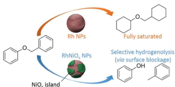
Fig. 23 Catalytic activity of NiO x /Rh NPs in the hydrogenolysis of the C–O bond in the lignin model compound. 291 (Copyright 2016 Elsevier.)
