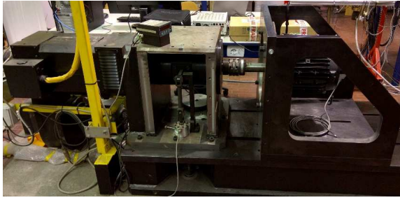
Fig. 10. Machine under test (right) and the driving machine (left)
