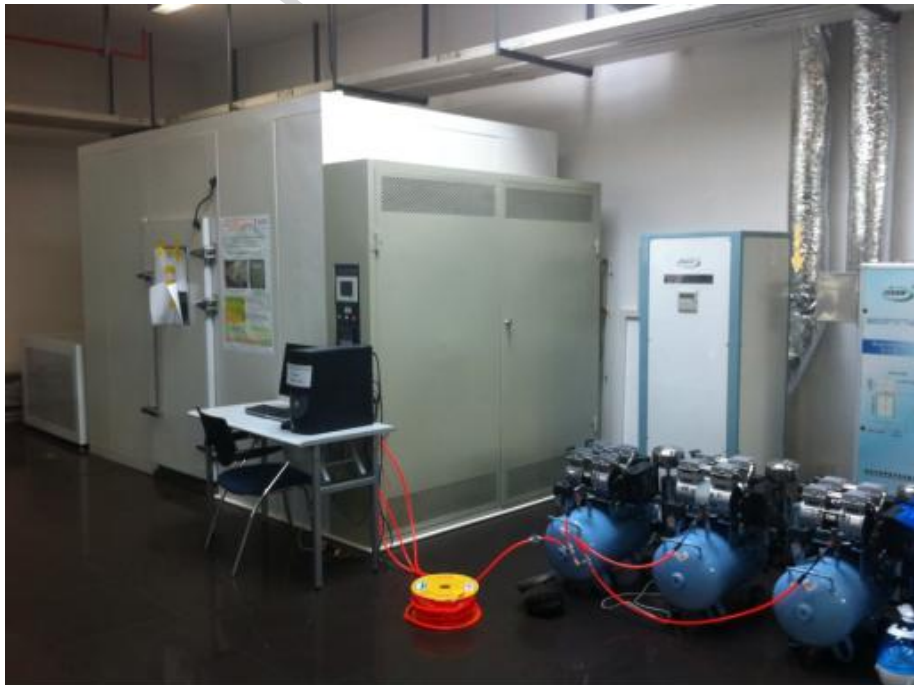
Figure 5 Experimental set-up with Edeson EWR-30S-A Environmental chamber
