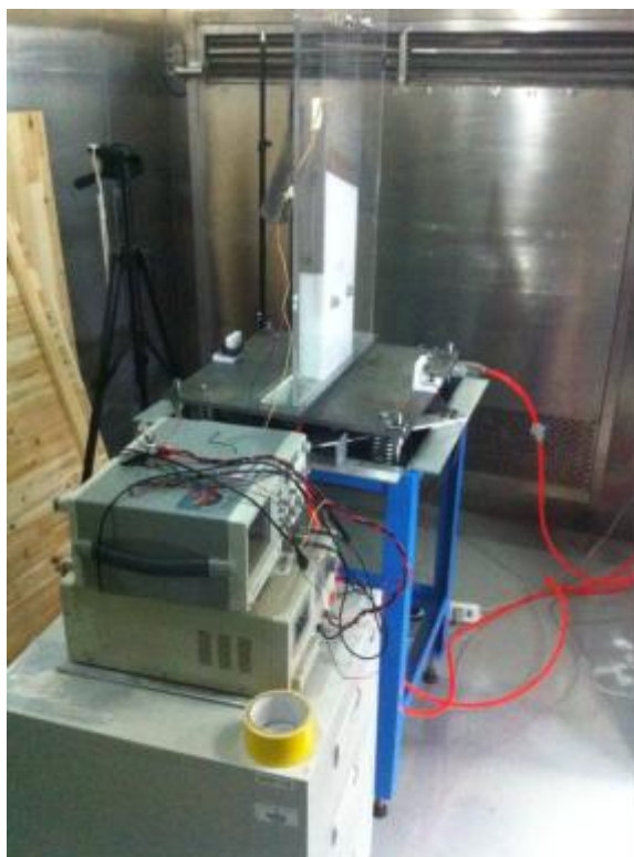
Figure 6 Vibratory separator in Edeson EWR-30S-A Environmental chamber
