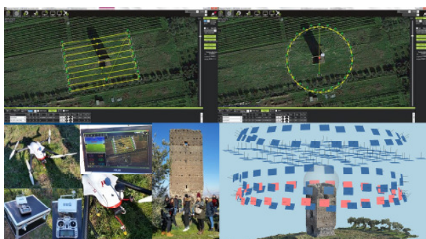
Figure 5. UAVs survey and PhotoScan final alignment
