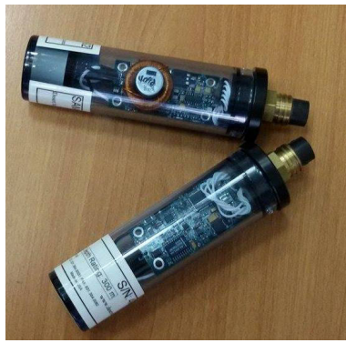
Figure 3.9: SAM-1 acoustic modem.
