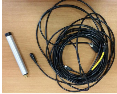
Figure 3.8: AS-1 hydrophone and Hydromic pre-amplifier.
