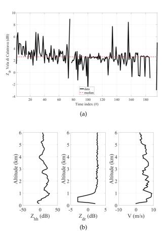
Figure 49: Monitoring of the differential reflectivity  $Z_{dr}$  on the 14th October 2015: (a) looking at the PSS (Vela di Calatrava); (b) looking at the vertical profile in ice above the radar (as in [57]) where V is the falling velocity in m/s.
