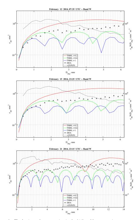
Figure 80: The horizontal cross section in the *W* band by comparing DDA computations (triangles) and TMM computations (dotted line). The product between the horizontal cross section and snowflake size distribution (red line) shows the main contribute of the particles with respect to the diameter disk-equivalent.
