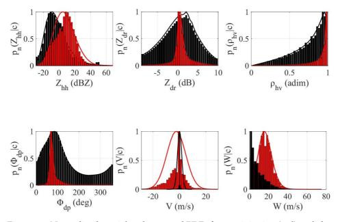
Figure 39: Normalized spatial and temporal PDFs for precipitation (red) and clutter (black) for the 0.5° elevation, 1 us pulse-length, 750 Hz PRF, 360° scans and 5 rpm obtained on data from 1 to 2 August. The bars represents the data selected in precipitation (red) and clutter (black), and the line represents the GEV-approximation. The method used to separate precipitation and clutter is a basic filter on the texture of the differential phase improved with the visual inspection of the data.
