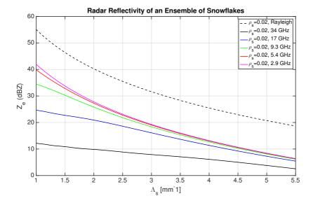
Figure 57: Reflectivities at different frequencies of an ensemble of snowflakes following the Rayleigh-Gans approximation at T = -10 °C for density of  $0.02 \text{ g/cm}^3$ : The Rayleigh-Gans approximation increasing the frequency (magenta, red, green and blue curves), and the Rayleigh approximation (dotted curve). Figure in [7].
