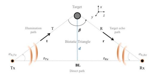
Figure 7: Bistatic geometry.
