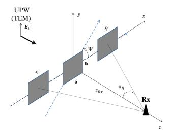
Figure 10: Simulated scenario and frame for the FSR model. The illuminated field is due to a uniform plane wave (UPW), transverse electromagnetic (TEM), that impinges on a rectangular shape target. It crosses the baseline moving from  $x_i$  to  $x_f$  with a uniform linear motion (constant velocity or zero acceleration).
