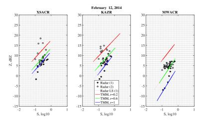
Figure 72: Case study: 12 February 2014 - Scatter plot of the equivalent reflectivities measured by the radar (points) with respect to the snow-rates S measured by PIP are shown. The pink line represents the Z<sub>e</sub>-S measured relationship evaluated using a least-square in the log-log space. Z<sub>e</sub>-S relations estimated with the TMM are shown for different aspect ratios (0.2, 0.6, 1) in red, green and blue lines.
