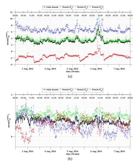
Figure 44: Temporal trend of acquisition of the mean value of the probability distribution for the co-polar reflectivity (a) and differential reflectivity (b).
