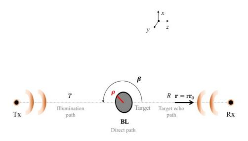
Figure 8: Forward scatter radar one-dimensional geometry.
