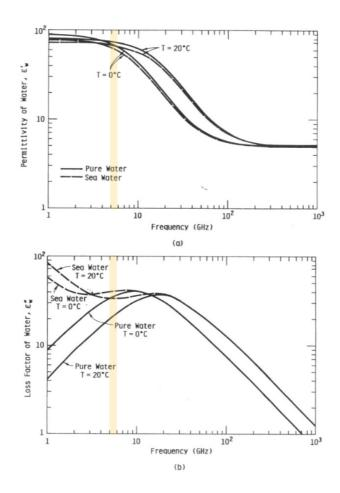
Figure 14: Complex relative permittivity of water: (a) permittivity; (b) loss factor. In yellow is highlighted the C band between 5 and 6 GHz. Figure from [21].
