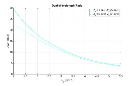
Figure 58: Dual-Wavelength Ratio (DWR) following the Rayleigh-Gans approximation at T =-10 °C for density of 0.02 g/cm<sup>3</sup>: DWR(S;K<sub>a</sub>) (cyan curve), and DWR(X;K<sub>a</sub>) (cyan dotted curve). Figure in [7].
