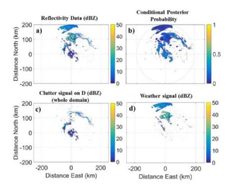
Figure 41: Case of study of the 5 August 2014 at the 17:10 UTC shown for the co-polar reflectivity  $Z_{hh}$  time frame: a) before and c, d) after the application of the Bayesian classification (**c** for the clutter signal on the whole domain **D** and d for the weather signal); in (b) the conditional posterior probability that is the argument of equation (134).
