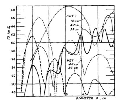
Figure 55: Values of  $10\log(Z_e)$ mm<sup>6</sup>m<sup>3</sup> corresponding to 1 gm<sup>-3</sup> of hailstones of uniform diameter D at three wavelength. Figure in [87].
