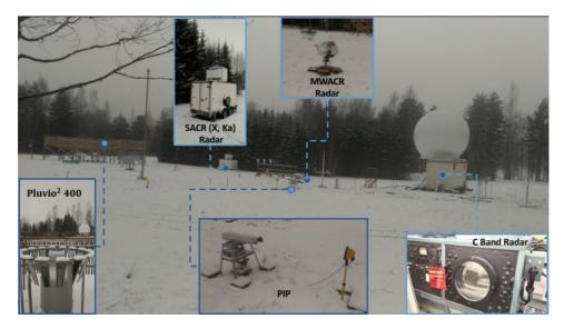
Figure 62: Measurement site shown with in situ and remote sensing instruments during the BAECC campaign 2014 at Hyytiälä, Finland.
