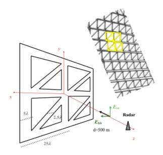
Figure 50: Geometry of the EM scenario represented by the PSS "Vela di Calatrava" element in the full-wave tool.
