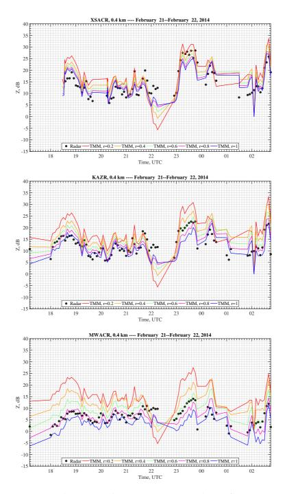
Figure 78: Case study: 21-22 February 2014 - Equivalent reflectivity measured by the radar (black points) compared with the TMM results for aspect ratios from 0.2-1.
