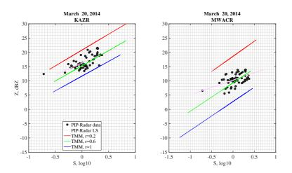
Figure 75: Case study: 20 March 2014 - Scatter plot of the equivalent reflectivities measured by the radar (black points) respect to the snow-rates S measured by PIP are shown. The pink line represents the  $Z_e$ -S measured relationship evaluated using a least-square in the log-log space.  $Z_e$ -S relations estimated with the TMM are shown for different aspect ratios (0.2, 0.6, 1) in red, green and blue lines.
