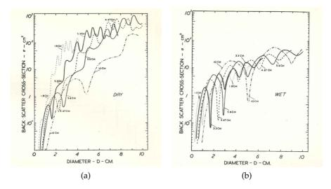
Figure 53: Back-scatter cross-section  $\sigma$  of spheres of ice with dry surfaces (a) and of liquid water (b), at the indicated wavelengths. Figures in [78].
