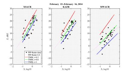
Figure 73: Case study: 15-16 February 2014 - Scatter plot of the equivalent reflectivities measured by the radar (black points) with respect to the snow-rates S measured by PIP are shown. The pink line represents the Z<sub>e</sub>-S measured relationship evaluated using a least-square in the log-log space. Z<sub>e</sub>-S relations estimated with the TMM are shown for different aspect ratios (0.2, 0.6, 1) in red, green and blue lines.
