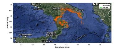
Figure 38: The clutter mask (red) shows the clutter scenario surround the radarsite of Mt. Pettinascura (green-point), the closest available radiosounding near Brindisi is also shown (green- cross). Background image from: Google Earth.
