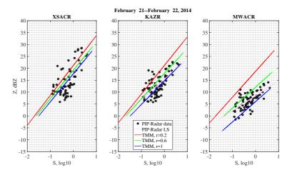
Figure 74: Case study: 21-22 February 2014 - Scatter plot of the equivalent reflectivities measured by the radar (black points) respect to the snow-rates S measured by PIP are shown. The pink line represents the  $Z_e$ -S measured relationship evaluated using a least-square in the log-log space.  $Z_e$ -S relations estimated with the TMM are shown for different aspect ratios (0.2, 0.6, 1) in red, green and blue lines.
