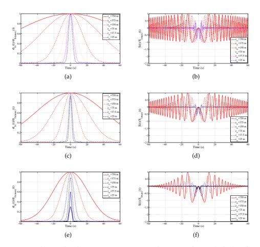
Figure 28: The circular shape signature is presented in terms of FS-CSs (a, b, c) and signal model (d, e, f), as the target/Rx distance  $z_{Rx}$  is varied, evaluated by equation (114). The area of the shape is the same for the rectangular target: (a, d) 2.4 m<sup>2</sup>, (b, e) 6.6667 m<sup>2</sup>, (c, f) 26.6667 m<sup>2</sup>. Diameters of the circle: 1.7481 m, 2.9135 m and 5.84 m. The Fraunhofer distances at f= 1 GHz are:(a, d) 20.3718 m, (b, e) 56.5884 m, (c, f) 226.3537 m.
