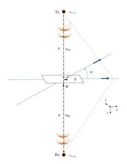
Figure 19: Geometry of FSR that takes into account the near-field condition with respect to both the transmitter and the receiver.
