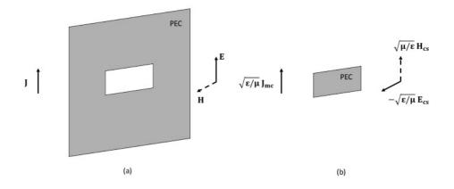
Figure 6: Babinet's principle applied to a screen (a) and a slot (b).
