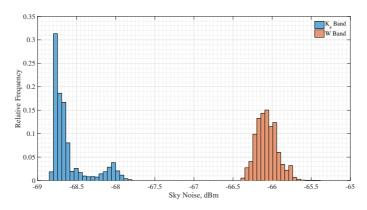
Figure 66: Relative frequency histograms of the sky noise for the Ka and W Band radars for all the ten days of BAECC IOP.
