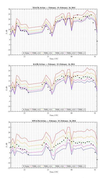
Figure 77: Case study: 15-16 February 2014 - Equivalent reflectivity measured by the radar (black points) compared with the TMM results for aspect ratios from 0.2-1.
