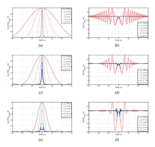
Figure 27: The rectangular shape signature is presented in terms of FS-CSs (a, b, c) and signal model (d, e, f), as the target/Rx distance  $z_{Rx}$  is varied, evaluated by equation (114). The area of the shape is: (a, d) 2.4 m<sup>2</sup>, (b, e) 6.6667 m<sup>2</sup>, (c, f) 26.6667 m<sup>2</sup>. Size of the rectangles along x-y:  $3 \times 0.8$  m,  $5 \times 1.33$  m and  $10 \times 2.67$  m. The Fraunhofer distances at f= 1 GHz are:(a, d) 60 m, (b, e) 166.6667 m, (c, f) 666.6667 m.
