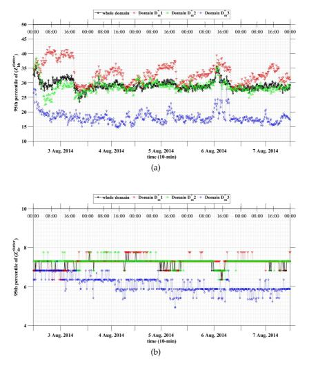
Figure 45: Temporal trend in time of acquisition of the 95th percentile of the cumulative distribution for the co-polar reflectivity (a) and differential reflectivity (b).
