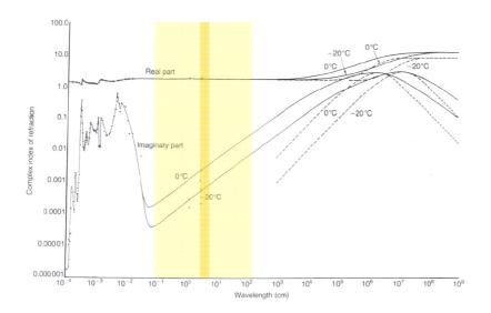
Figure 17: Complex relative permittivity of ice from [31]. In orange is highlighted the C band between 5 and 6 GHz. The yellow area indicates a much larger range between 0.3 and 300 GHz.
