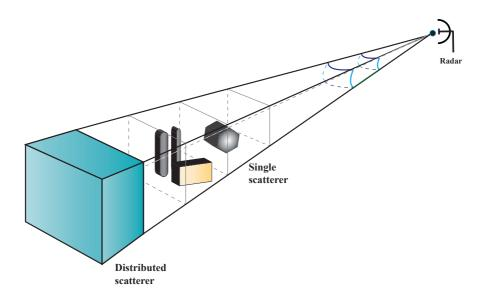
Figure 2: Single and distributed scatterers inside the radar beam.
