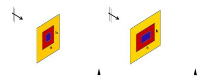
Figure 31: Simulated FSR scenario to investigate the effects of the target dimension and shape. Three different square (left) and a rectangular (right) metallic plates are considered. Squares size along x-y: 1 (blue), 3 (red), 4 (yellow); rectangular size along x-y:  $2 \times 1$  (blue),  $6 \times 3$  (red),  $8 \times 4$  (yellow).
