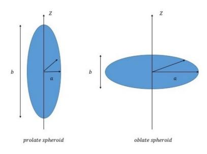
Figure 15: Spheroids described in terms of aspect ratio (r = a/b): prolate (r < 1), oblate (r > 1). The spherical shape not shown is for r = 1.
