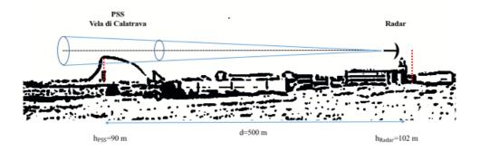
Figure 46: Radar clutter scenario considered: C-band Doppler dual-polarization Polar 55C located South-East of Rome (Italy) and the permanent scatterer used for the study, that is named Vela di Calatrava.
