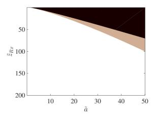
Figure 26: Map of the area where the phase error does not exceed  $\pi/8$  (i.e., threshold  $\pi/8$  applied to the maps of Figs. 24 and 25). The black and pink areas refer to the values in which the first-order model exceeds the threshold and only black in which the second-order model exceeds the threshold.
