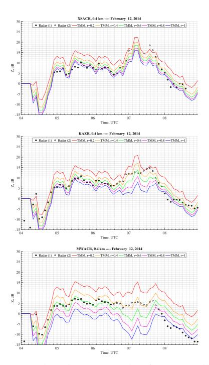
Figure 76: Case study: 12 February 2014 - Equivalent reflectivity measured by the radar (black points) compared with the TMM results for aspect ratios from 0.2-1.
