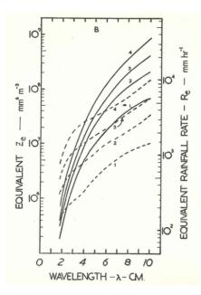
Figure 54:  $Z_e$ , the equivalent Z, of the four exponential hail spectra, as a function of wavelength. On the right is a scale of equivalent rainfall rate  $R_e$ , derived from the empirical relation:  $Z = 486R^{1.37}$  [86]. Figure in [78].
