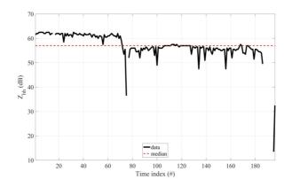
Figure 48: Monitoring of the reflectivity factor  $(Z_{hh})$  looking at the PSS (Vela di Calatrava) on the 14th October 2015. A de-pointing is clearly visible around the 75<sup>th</sup> daily-time index.
