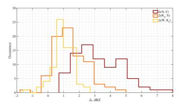
Figure 64: Calibration error histograms relates to the differences ( $\Delta$ ) between: X and C band radars (dark red), Ka and X band radars (orange), and W and Ka radars (yellow).
