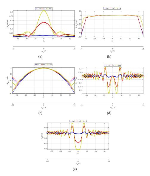
Figure 32: Scattered ('S') and total ('T') signals vs. target horizontal position, collected by the receiving antenna for three different square PEC objects as in Figure 31: side 1 (blue), 3 (red), 4 (yellow). (a) Scattered-field amplitude; (b) Scattered-field phase difference; (c) Scattered-field unwrapped phase; (d) Total-field amplitude; (e) Total-field phase. Closed-form results (solid) and full-wave CAD (dots) are compared.
