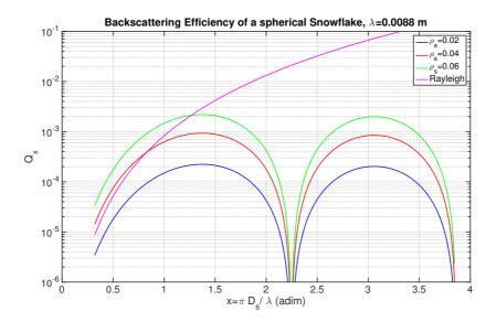
Figure 56: Backscattering efficiency of a snowflake Q as a function of size parameter x for different snow densities in  $K_{\alpha}$  band at T = -10 °C: The Rayleigh-Gans approximation (green, red and blue curves), and the Rayleigh approximation (magenta curve). Figure in [7].
