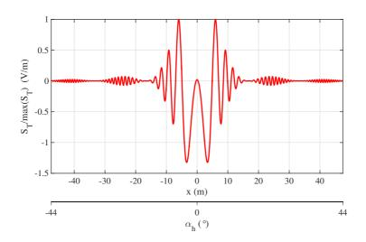
Figure 11: Amplitude of the total signal (equation (69)) collected by the receiver for a square metallic object horizontally moving in the far-field with respect to the receiver having size  $a = b = 3\lambda$ . The distance object-Rx  $z_{Rx} = 50\lambda$  for a  $\lambda = 0.5$  m.
