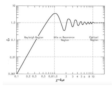
Figure 3: Backscattering efficiency as a function of a dimensionless size parameter  $\chi$ , useful to highlight the three domains of scattering [21].
