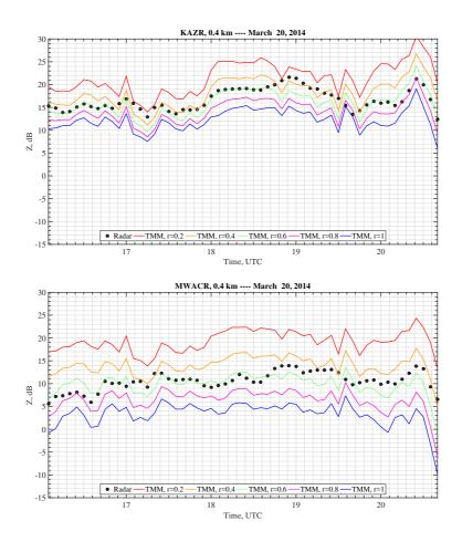
Figure 79: Case study: 20 March 2014 - Equivalent reflectivity measured by the radar (black points) compared with the TMM results for aspect ratios from 0.2-1.
