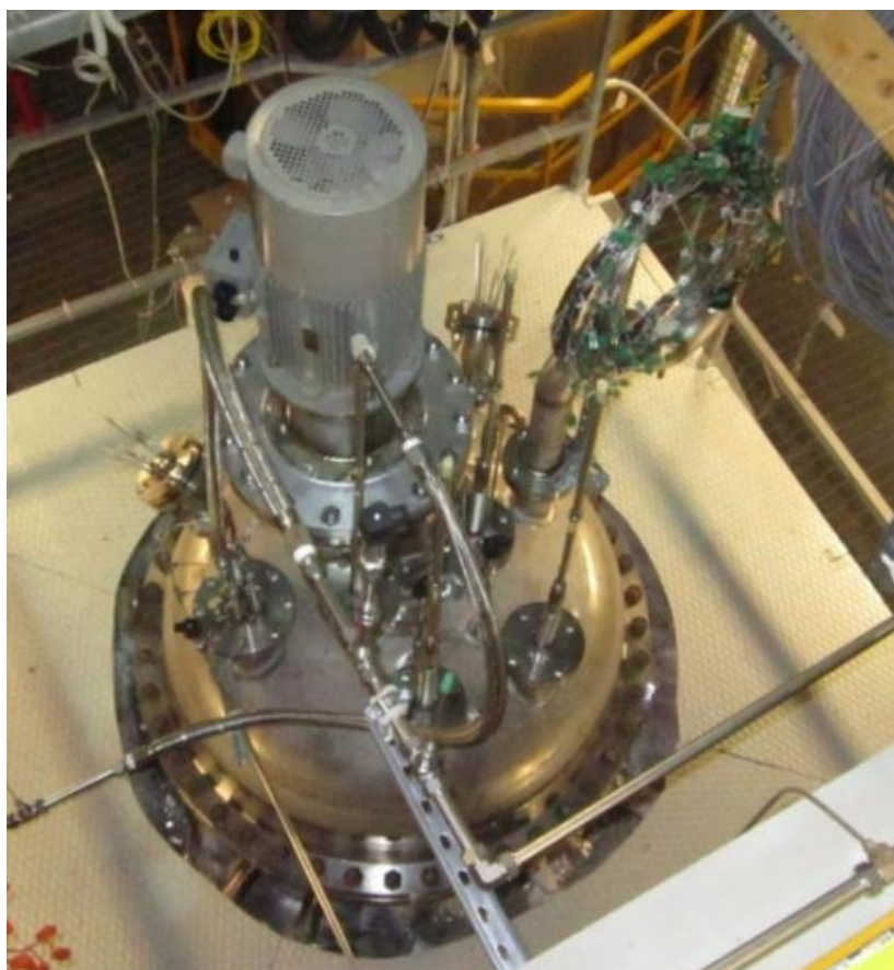
Figure 17: CIRCE Cover. MAXSIMA test section
