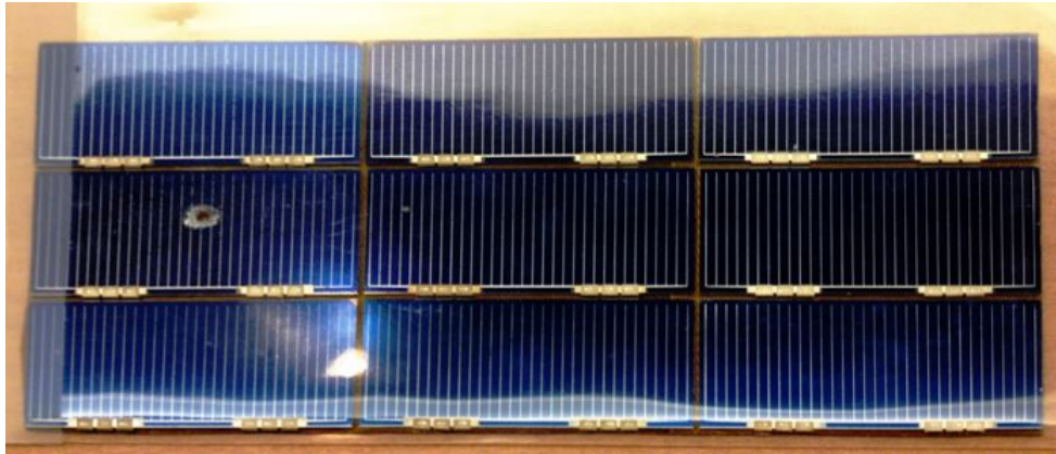
FIGURE 1.1: ESA built-solar cells retrieved from the Hubble Space Telescope in 2002.
