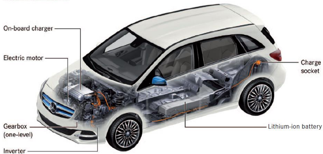
Figure 2-1: Electric drive components of the B-Class Electric Drive
