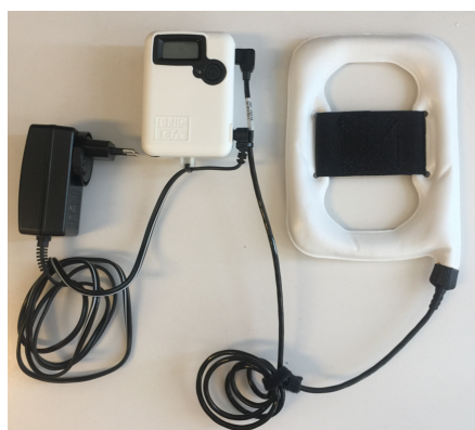
Figure 5.8: I-One coil exposure setup with the generator, the power supply and the solenoid.
