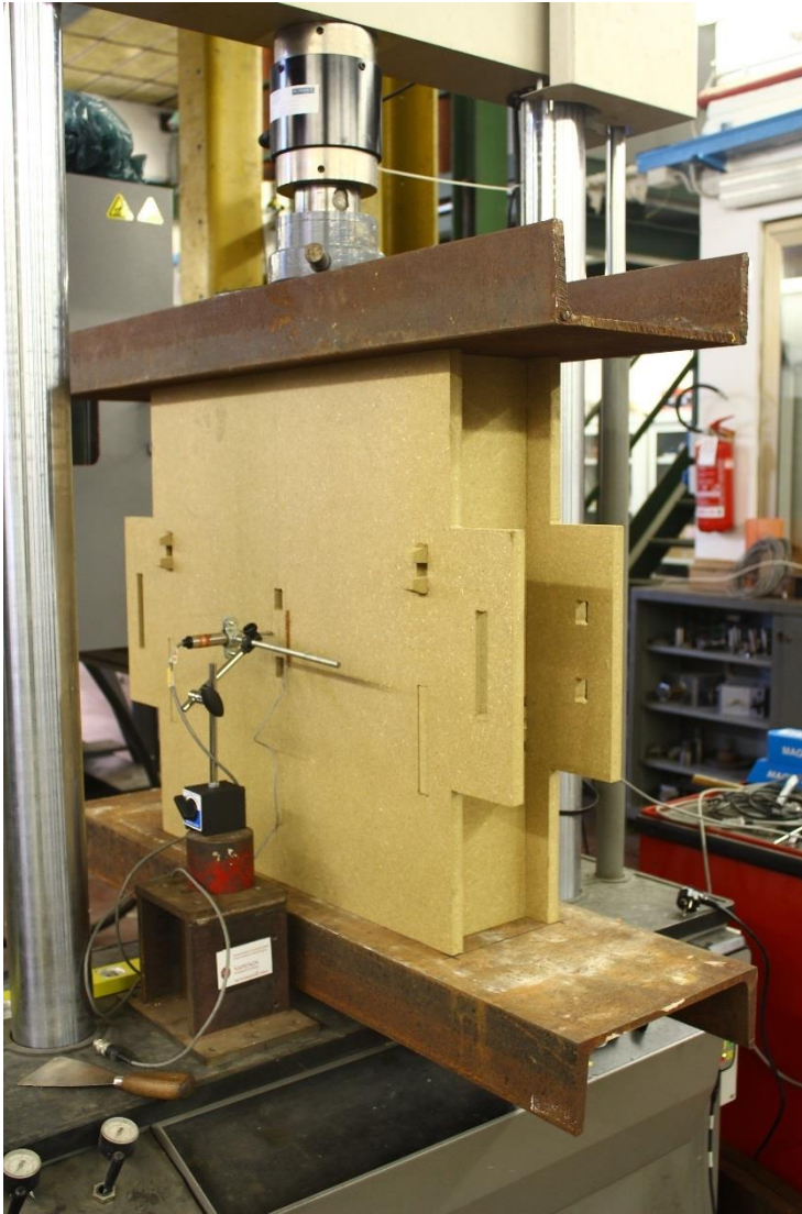
Figure 6-18: Step (3) Complete test setup where a 300 UPN profile is placed above test piece with manual alignment to center of upper loading cell. Two 60 mm strain gauges were attached on both sides at central zone of sheathing panel leaving an offset of 5 mm from central key insert hole.
