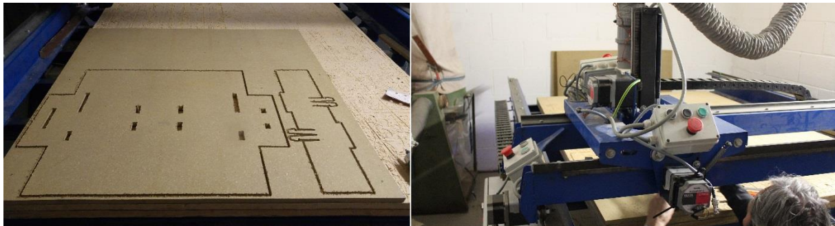
Figure 6-5: CNC milling of the final prototype parts
