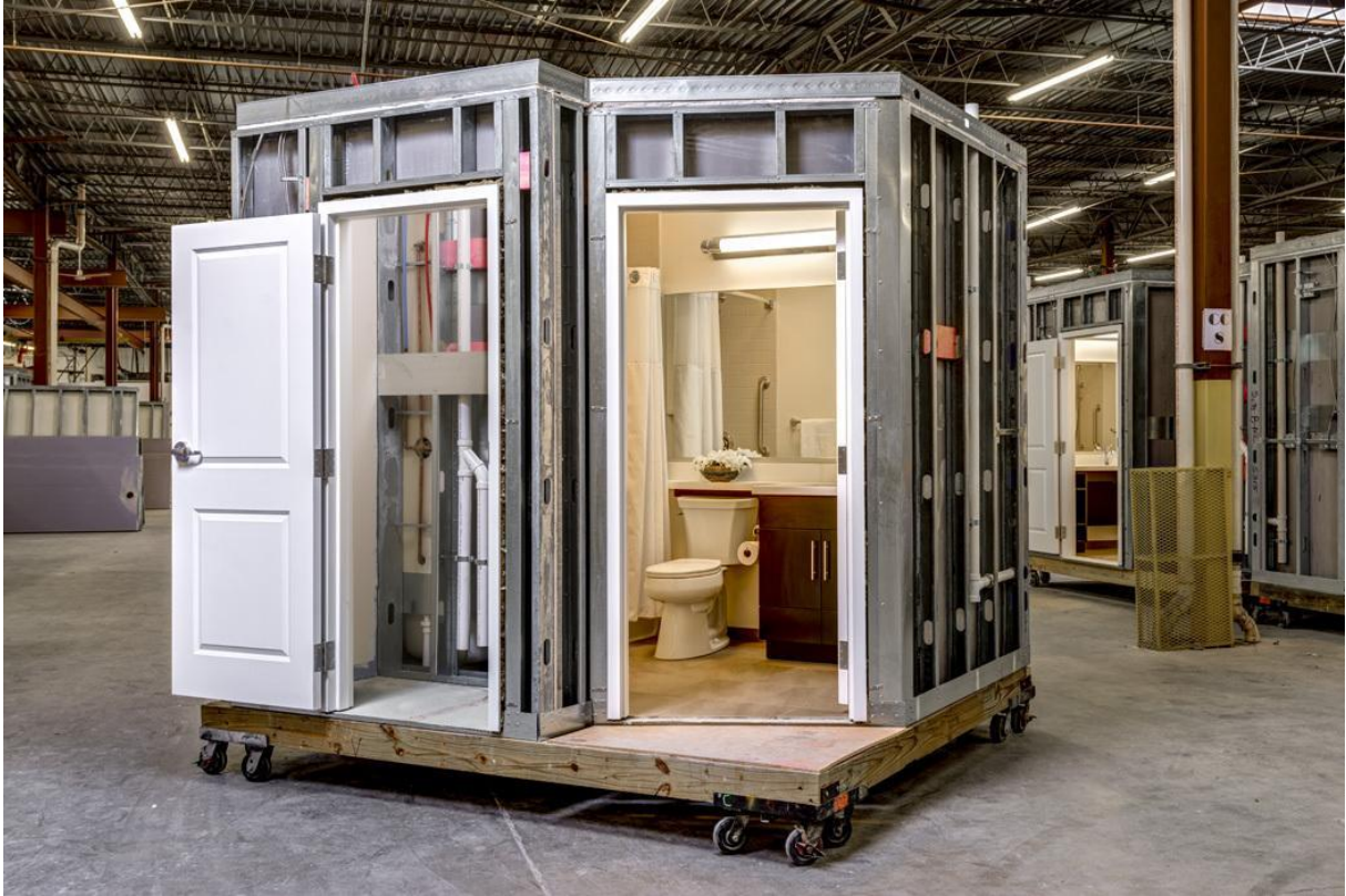
Figure 4-2: Prefabricated bathroom pod manufactured by PIVOTEK, an American company specialised in off-site prefabricated bathroom pods for housing and hospitality. Source: Pivotek LinkedIn post.
