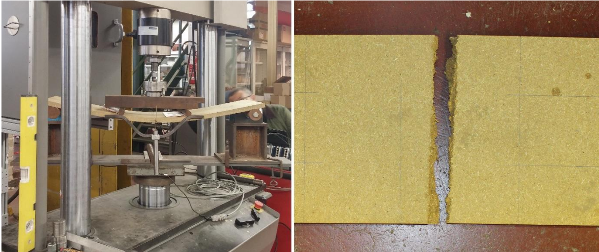
Figure 4-12: (Left): 4-point bending test setup. (Right): Brittle Material Failure in both test pieces.
