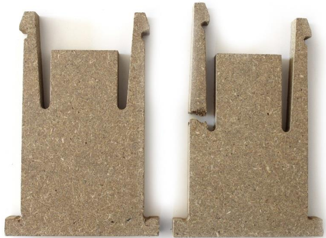
Figure 5-14: Numerous snap fit arms were fabricated and manually tested for ease of assembly and disassembly. (Left) short cantilever arm (76 mm), (Right) Long cantilever arm (90 mm) that was easily broken.
