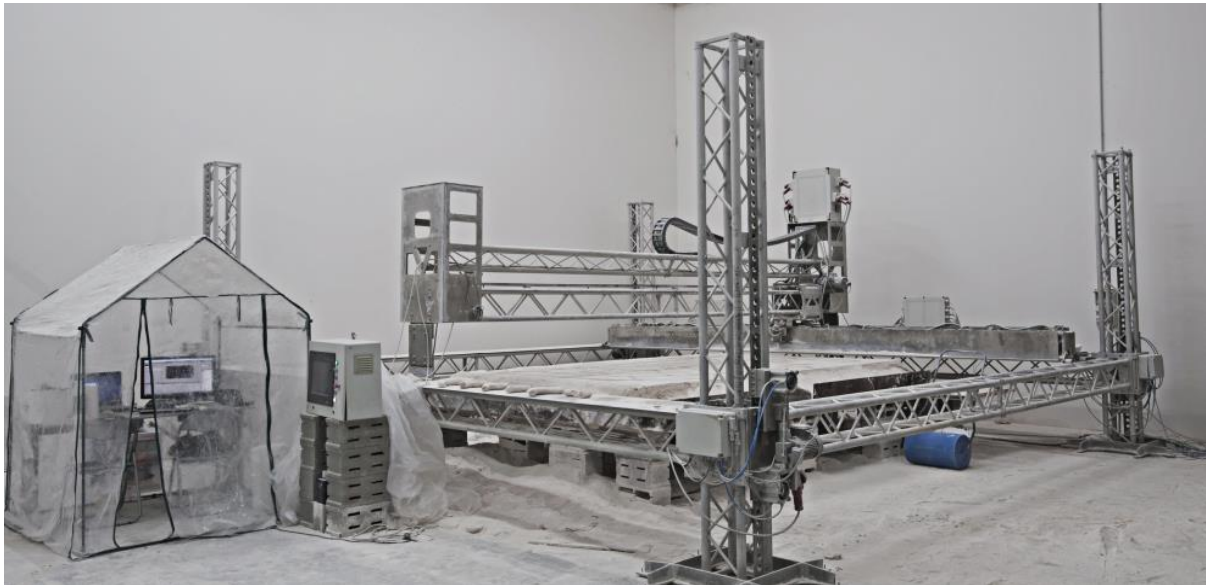
Figure 2-16: D Shape 3D printing Technology developed by Enrico Dini. Source: https://d-shape.com/
