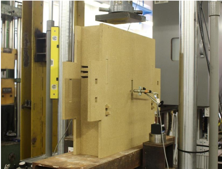
Figure 6-17: Step (2) Test piece placed on lower base and two LVDT measuring equipment are placed on both sides of test piece on magnetic bases.
