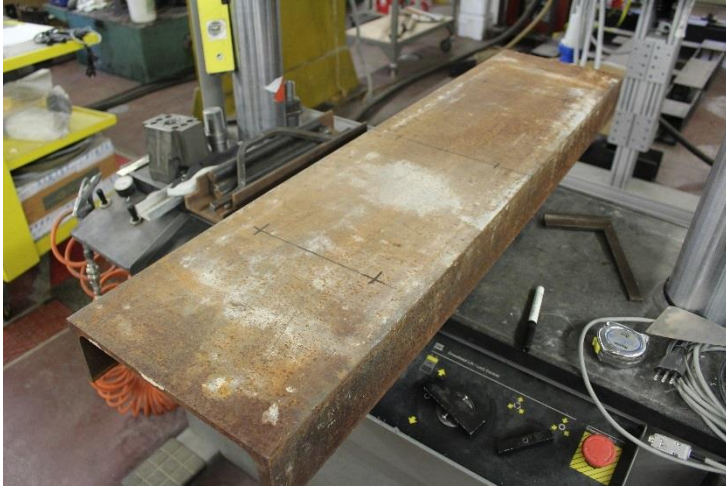
Figure 6-16: Step (1): UPN 300 profile placed on lower MTS piston and used as support base for test piece. The test piece was aligned to center of UPN profile in both directions in order to maintain symmetry of load distribution.
