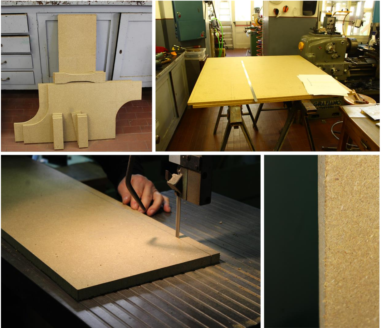
Figure 8-3: Test piece preparation, cutting and final edge condition
