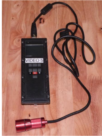
Figure 2. The V.I.O. Point-of-View video camera used in the Helmet-CAM, showing the body of the camera and the lens component (below the body) attached by cable.
