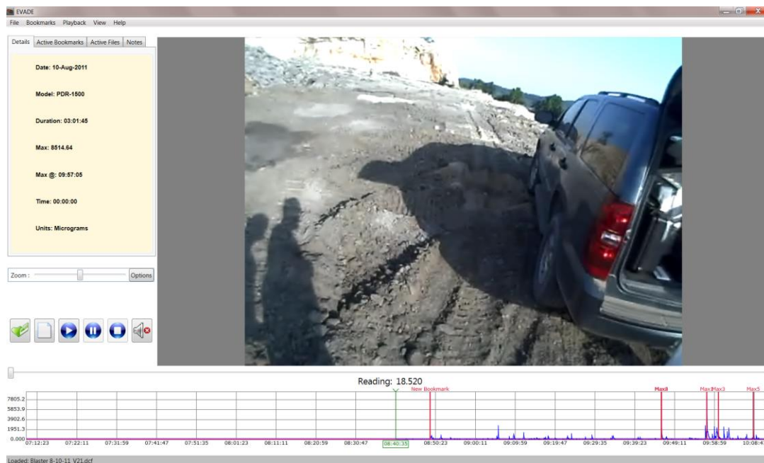
Figure 19. The EVADE main window after an existing dust exposure analysis is selected through the Open command.
