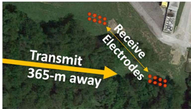
Fig. 9. Satellite image of the receive area. The orange dots indicate a single ground rod's location. A cluster of dots represents one electrode.
