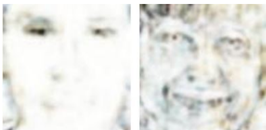
Figure 10: Local SSIM of the images used in Figure 9. The darker areas represent the least structural similarity between Bicubic with ANN and Bicubic only, while the white areas represent the most structural similarity. Areas of smoother details are similar in both images, as can be seen in the smoother skin around the cheeks. However, areas with finer details like eyes, teeth, wrinkles and hair are structurally dissimilar- implying a greater improvement in these areas of the image obtained by the Bicubic with ANN.
