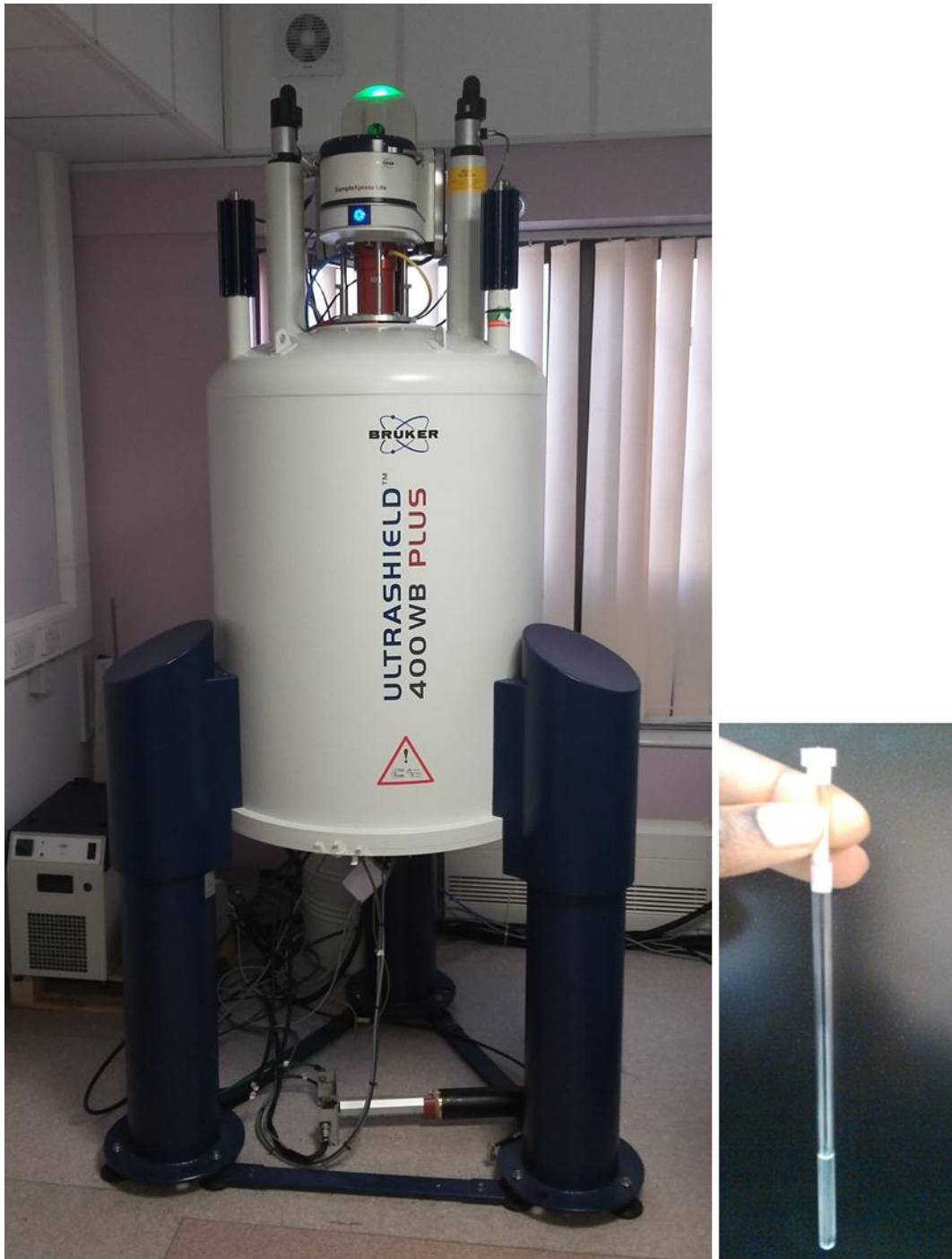
Figure 2.2. A 9.4T (400 MHz) Bruker Avance III MR spectrometer and 5mm BBO broadband Observe probe (left), and MR 5 mm glass tube containing cervicovaginal fluid sample (right).
