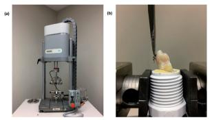
**Fig. 2:** (a) Instron testing machine with sample held in position. (b) Instron attachment blade placed at the bracket ligature groove ready for testing at a crosshead speed of 1mm/min.
