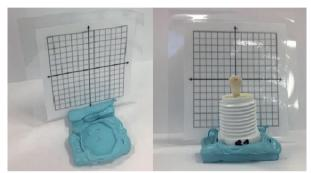
Fig. 1: Mounting jig for standardization of 45° rotational movement.
