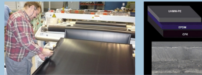
Fig. 5: Producing of the slide-foil and layer structure (Source: PerLaTech)
