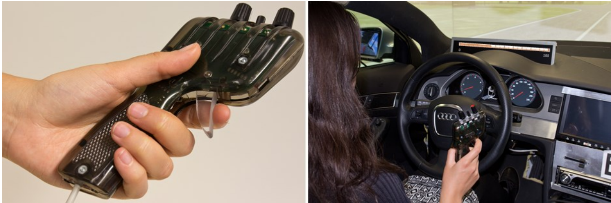
Figure 13. Handset control (left) for the online assessment of comfort while driving highly automated in the driving simulator (right).
