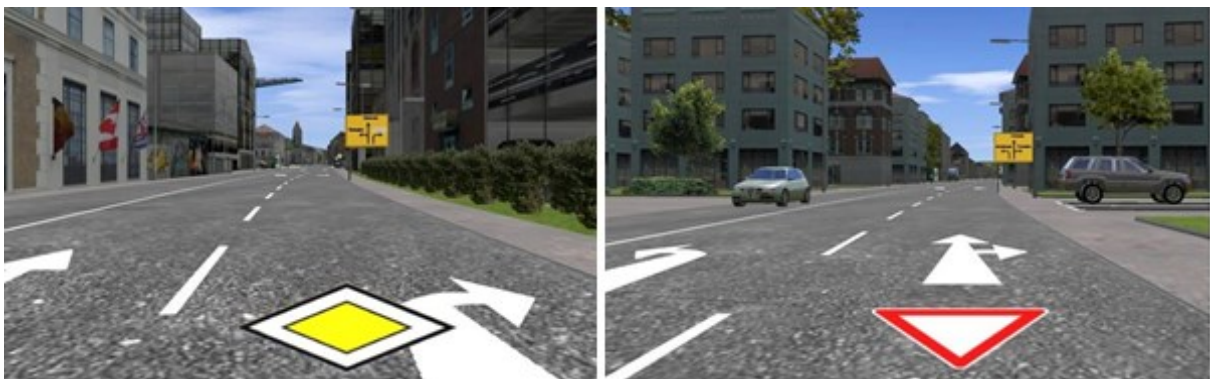
Figure 10. Simulated Augmented Reality Display 150 m in front of an intersection where the driver (a) has the right of way or (b) has to yield right of way.
