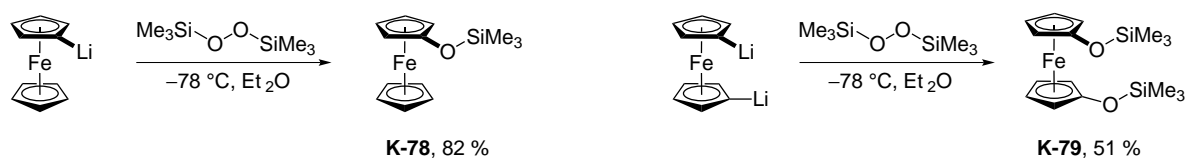
Figure 2.44 Oxygen functionalization of ferrocenes with bis(trimethylsilyl)peroxide. [158,159]
