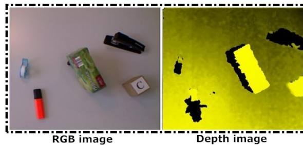
Fig. 1.37 Produced images by Kinect sensor
