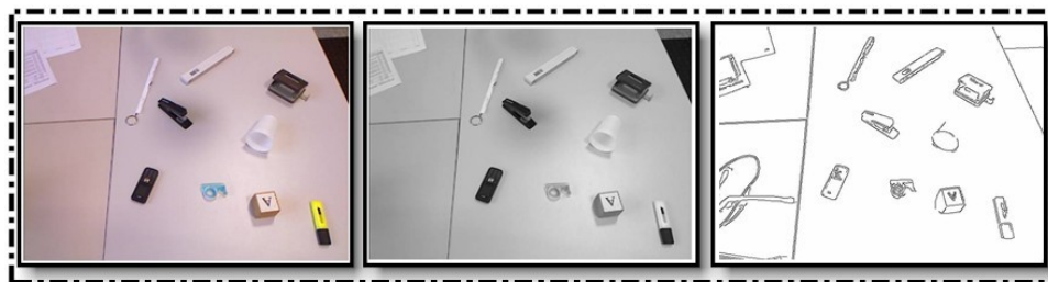
Fig. 2.18 Converting from RGB to binary image
