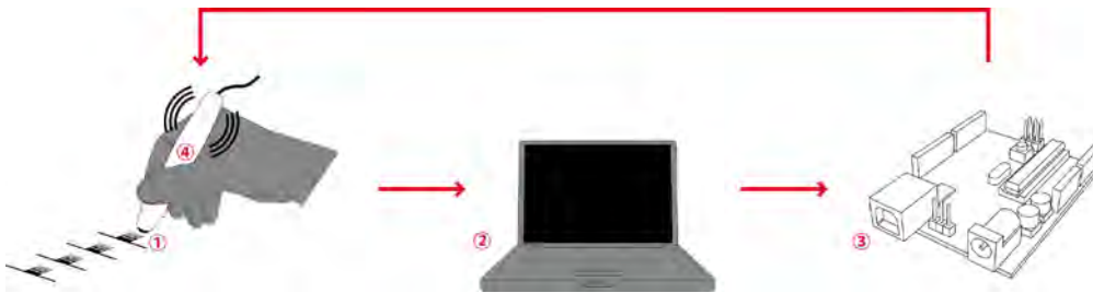
Figure 2: 1) Position tracking; 2) Processing of effect strength on the personal computer; 3) assignment of the arduino board to 4) control the actuators in the stylus.
