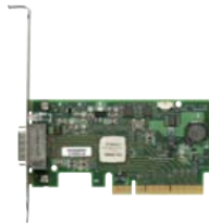
Figure 1.11: Mellanox InfiniHost III Lx HCA (taken from [3])
