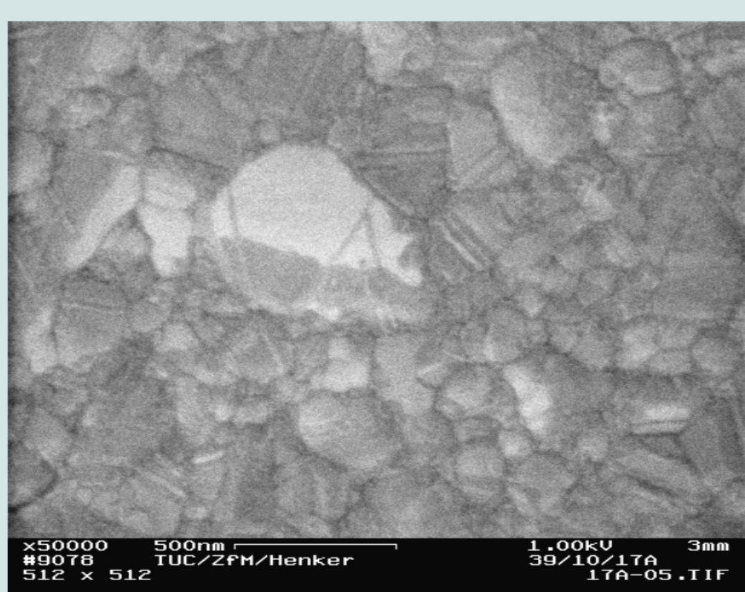
Fig. 1: SEM micrograph of CVD copper deposited by BUTFA on a sputtered Cu seed layer at 300 °C.
