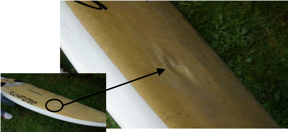
Fig. 7 Surface fracture damage due to impact load
