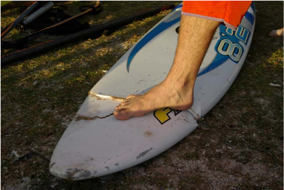
Fig. 8 Complete nose damage due to impact load
