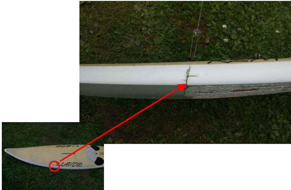
Fig. 19 Complete bottom fracture due to hard nose dive
