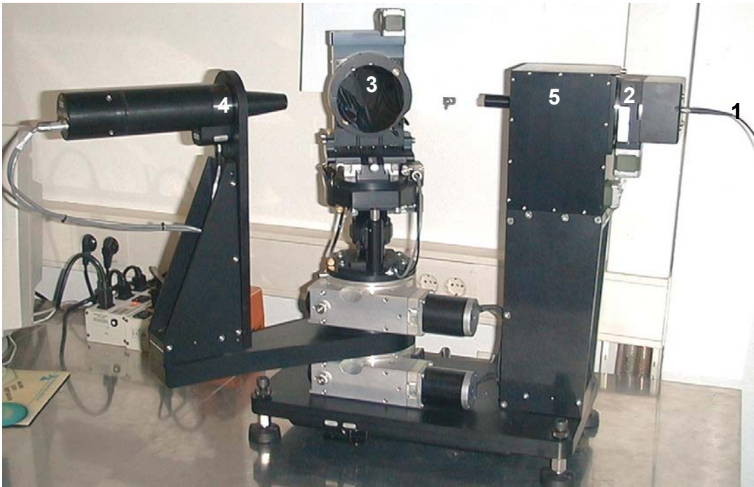
Fig. 3.14. Woollam VASE Ellipsometer. Optical fiber (1), polarizer (2), sample (3), analyser (4) and autoretarder (5) are marked on the picture by numbers.
