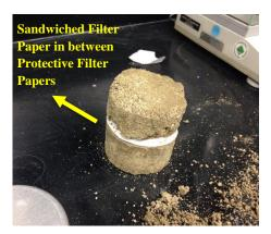
Figure 4.3 Soil Specimen Prepared for Matric Suction Measurement
