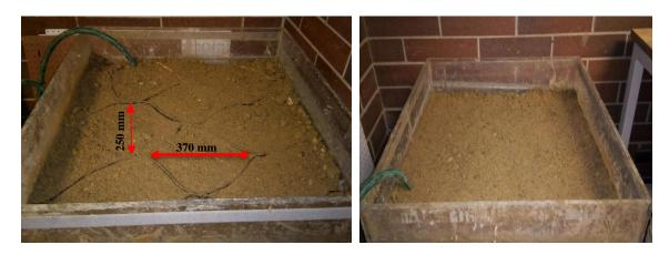
Figure 3.20 Geocell Placement
