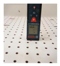
Figure 3.8 Laser Distance Measuring Tool
