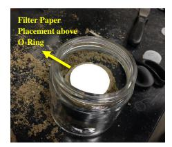
Figure 4.4 Soil Specimen Prepared for Total Suction Measurement
