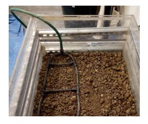
Figure 3.15 Placement of Soaker System at the Top Half of Subgrade
