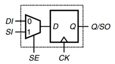
Figure 1.1: A Typical SCAN Cell [7]
