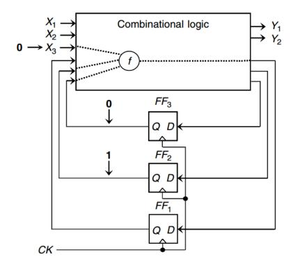
Figure 2.3: Testing a Normal Sequential Circuit for Fault, f [7]
