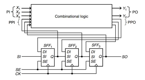
Figure 1.2: Mux-D Full SCAN Circuit [7]
