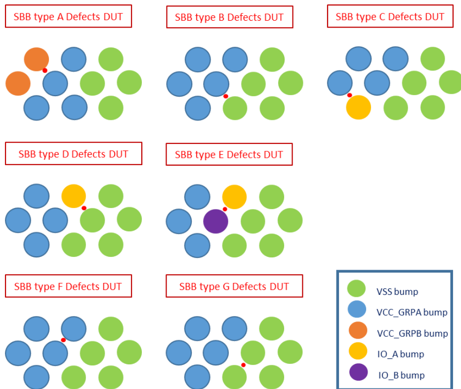
Figure 2.7: Types of SBB defects.
