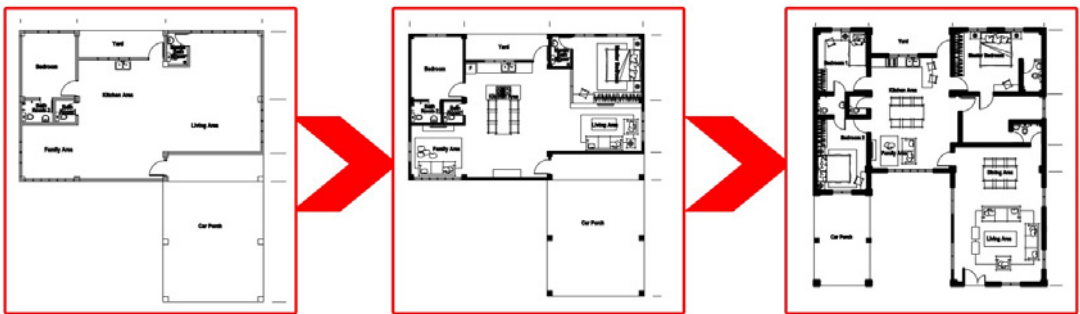
Figure 1: Evolution of house renovation using flexible floor plan with sustainable inner wall.
