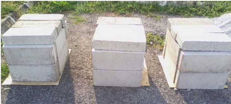
Figure 1. Model design of concrete block made from concrete waste mixture
