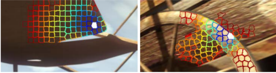
Figure 4.2: Two examples of support neighbours ( n = 100 ). The support neighbours are represented by color with blue meaning they are closer and red meaning they are farther away from the white superpixel seed. The distance is calculated via a geodesic approximation, as in EpicFlow. Figure from [HLS17].
