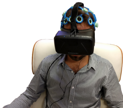
Figure 6.4: A participant using the Oculus Rift together with earphones and the Ultracortex.
