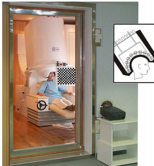
Figure 2.8: A typical MEG sensor. The white container-like looking device contains several sensors which allow the measurement of magnetic activity triggered by neurons [HHI + 93].
