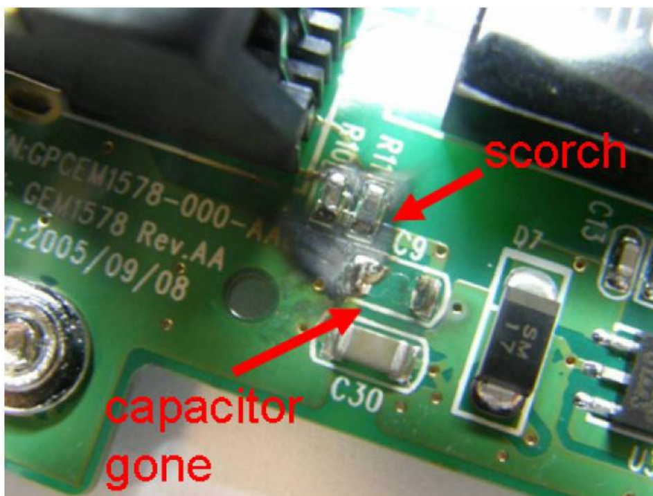
Figure 4: SCADA Circuit Board Capacitor Damage from Pulse Testing 46
