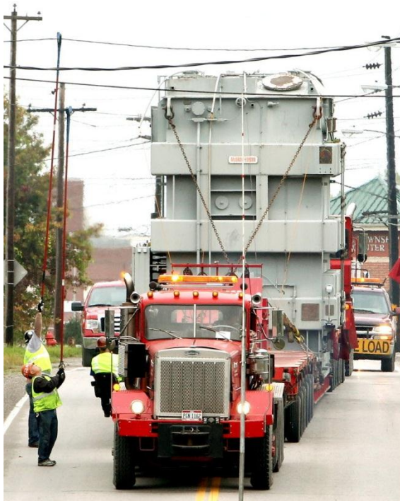
Figure 15: Nuclear Plant Step-up Transformer Being Transported through Ohio 131
