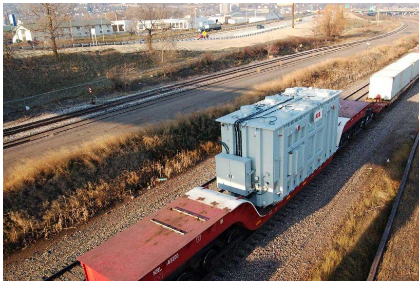
Figure 16: Transformer on Specialty Rail Car 132
