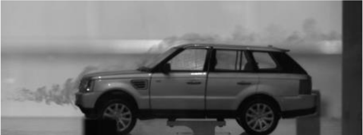
Figure 29. Smoke flow visualization
