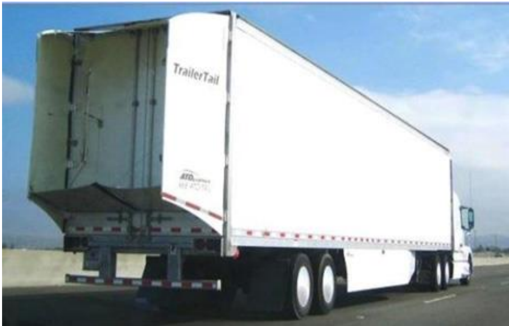
Figure 7. 18-Wheeler truck fairings and side air dams
